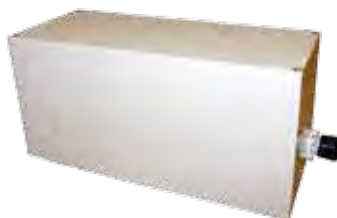
BSF-1030-1090/1347 Bandstop Filter for Link16 frequencies
